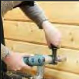
The ALLMAT multi-purpose hole saw has sharp toothing for excellent quality cutting with fast advance. The teeth will last if you take care of the hole saw and use it on the materials for which it is intended. If the teeth are no longer as sharp as they were due to extended or inappropriate use, you can have them resharpened by your sharpening service.
